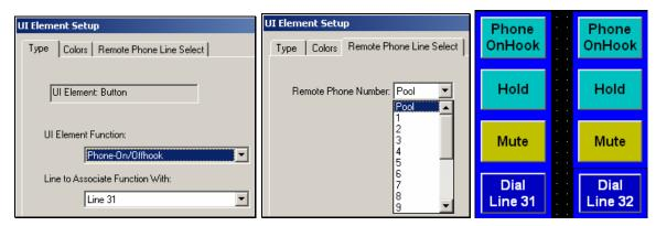
Figure 6 C-Soft Phone Control Buttons Setup
